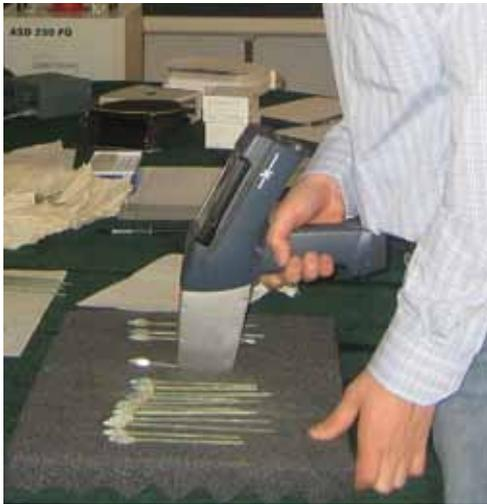
**Fig. 9:** Analysis of bronze weapons using a portable XRF.
