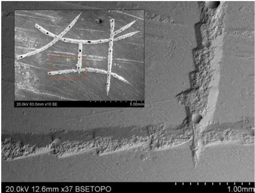
**Fig. 11:** SEM image showing a detail of a character of an inscription on a weapon surface, showing the triangular chisel marks forming the lines, with (inset) SEM overview of the character; both images are from a silicone rubber impression so that they show a positive cast of the inscription, with protrusions representing depressions on the weapon itself.
