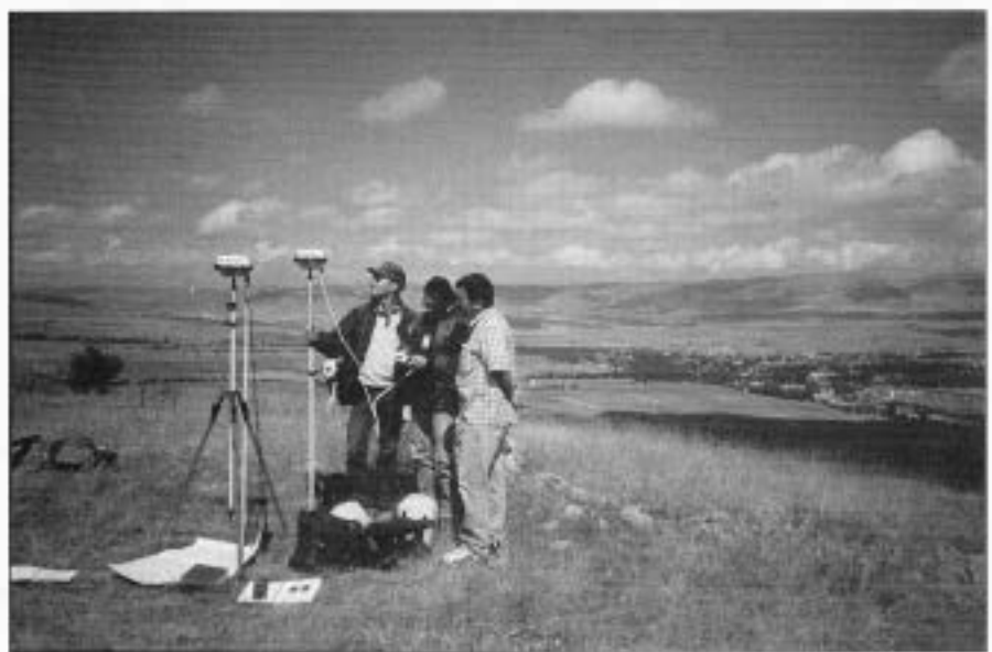
Figure 2 Setting up for survey of a hilltop site using the GPS (Global Positioning System) technique.
